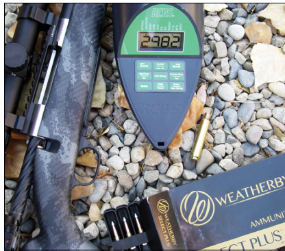
Factory 6.5 Weatherby RPM ammunition chronographed just under 3,000 fps using Nosler 140-grain AccuBond bullets.
