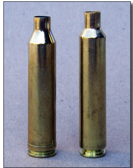
The 6.5 Weatherby RPM case (right) has slightly less powder capacity than the .264 Winchester Magnum (left). Note the 35.25-degree shoulder angle of the 6.5 RPM.
